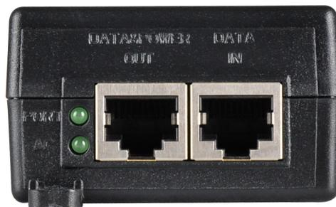
Ruijie RG-E-130 Power Injector RJ-45 Ports
